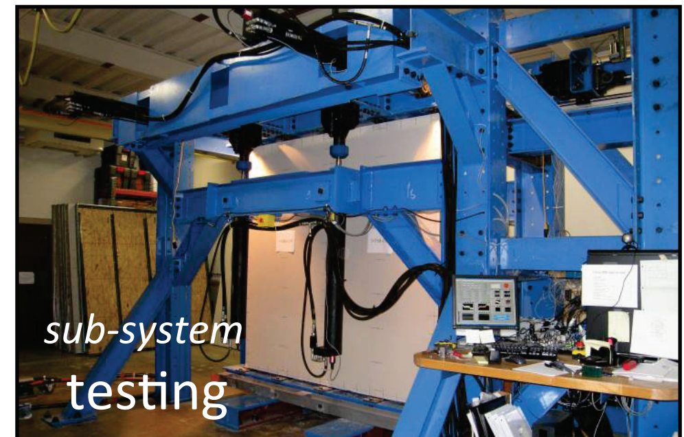
Figure 1 Schematic of proposed testing (a) sub-system tests of EXP-1, and system interaction testing of (b) a wall line with gravity and shear walls, EXP-2, and (c) a shear wall with floor detailing included, EXP-3
